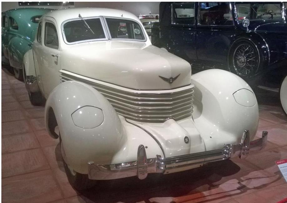
Finally, a rare sight in Britain even in its 1936 hey-day was this Cord Beverley. With its 4730cc Lycoming engine the Beverley was the first American production saloon to achieve a genuine 100mph. Its advanced design incorporated retractable headlights, an electrically operated gearbox with pre-select gear change was ahead of its time and the buying public were not persuaded. In addition early teething troubles led to production ceasing after only 2,320 had been produced.
